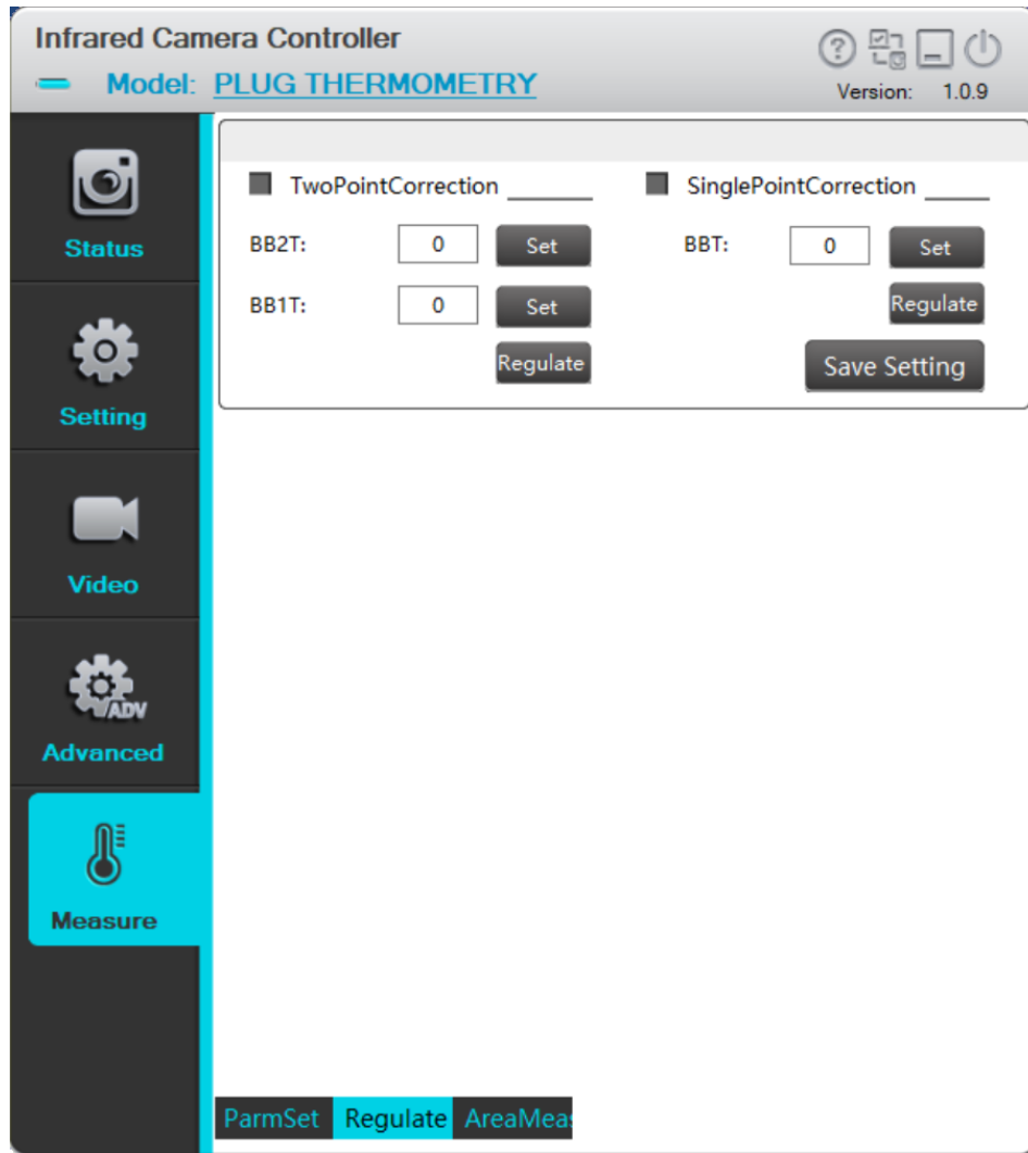
Fig.4-31 blackbody correction interface
