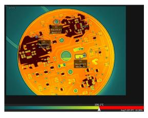
③ In-interval isotherm E: the in-interval isotherm button of infrared video or infrared image. After clicking, you can fill in the values of the lowest temperature and the highest temperature, and set the temperature range. As long as the temperature values of the pixels on the infrared image are within the lowest and highest temperature ranges, the colors in this area will be displayed in the corresponding colors.
