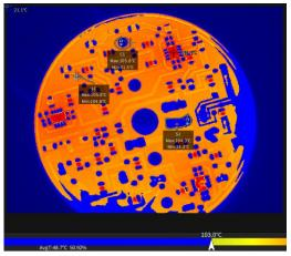
② High isotherm 1: the high temperature isotherm button of infrared video or infrared image. After clicking, you can fill in the value of the highest temperature and set the temperature range. As long as the temperature value of the pixel on the infrared image is above the highest temperature range, the color of this area will be displayed in the corresponding color.
