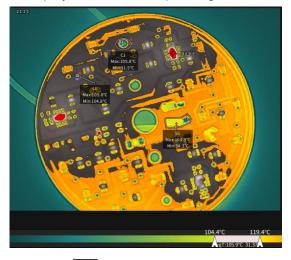
④ Out-of-interval isotherm E: the out-of-interval isotherm button of infrared video
