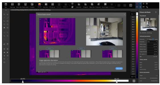
Select the "first position point": left click to select the position in the infrared thermal image, and then select the position corresponding to the same target in the visible light image.
