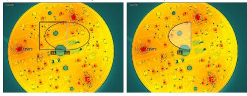
Difference Set. First, select an area object, click the Difference Set icon, and then select the area object to perform the Difference Set operation to generate a combined object.
