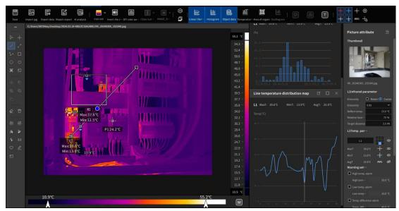
This software supports multiple categories of thermal images for secondary analysis, including analysis object DIY, image dimming (mix/straight/linear), LevelSpan dimming, temperature measurement parameter correction, 3D/straight/linear temperature image, etc.
